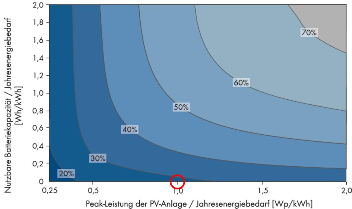
$$\frac{\text{Peak } 5'000 \text{ Wp}}{\text{Bedarf } 5'000 \text{ kWh}} = 1 \text{ Wp/kWh}$$
